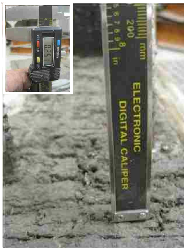
Figure 3.10. Surface roughness measurement
