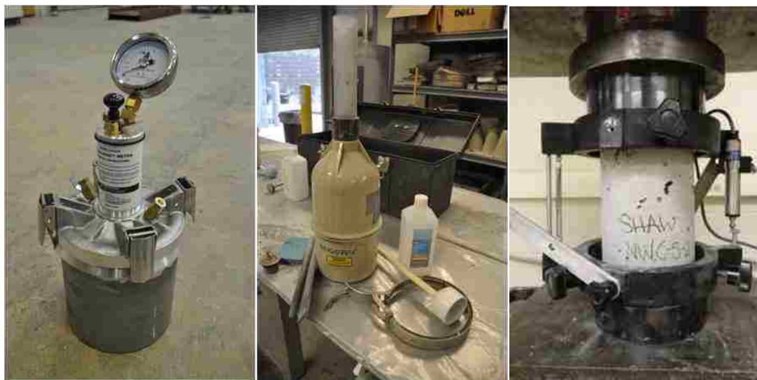
Figure 3.4. Pressure meter, volumetric meter, and modulus of elasticity yoke (from left to right)
