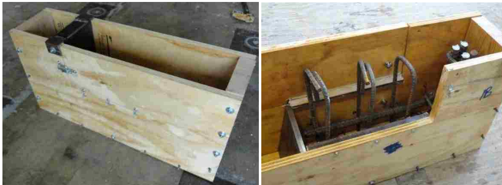
Figure 3.8. Test specimen formwork
